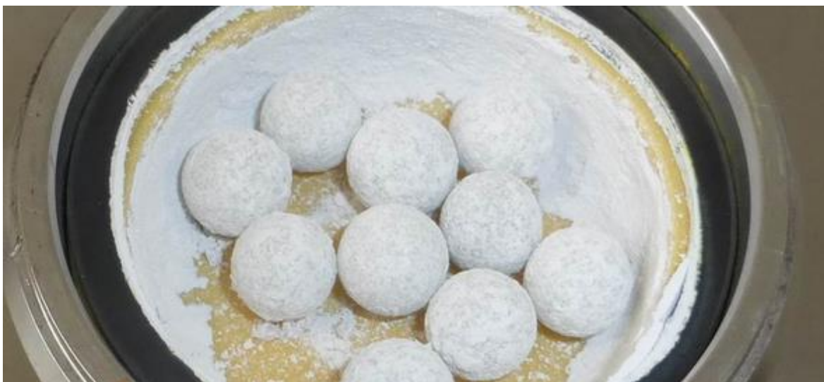
After only one minute of dry grinding, sample is already sticking to bowl and grinding balls. Longer dry grinding is not possible to improve fineness significantly.
