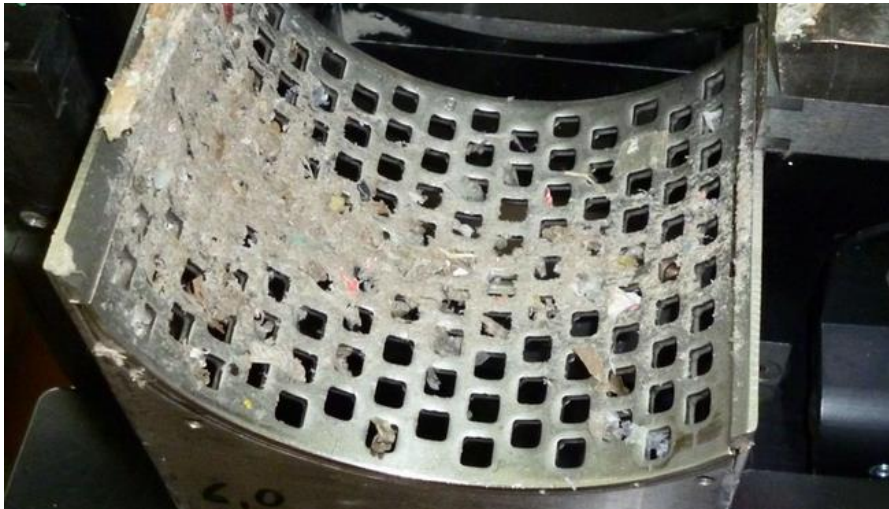
Melted sample started sticking to the 6mm sieve cassette.
