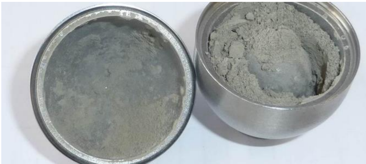
Sample after 1 minutes of grinding: sample is already sticking lightly to bowl and grinding ball.
