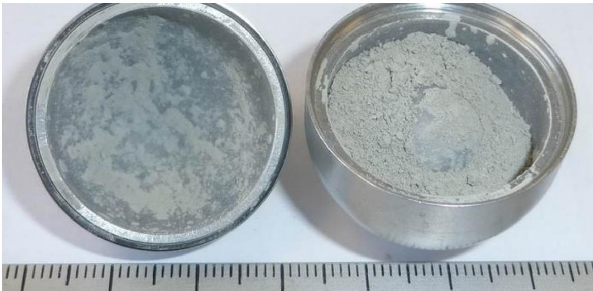
Sample 2710 is also sticking after 1 minute of grinding. Sample can still be brushed out easily.
