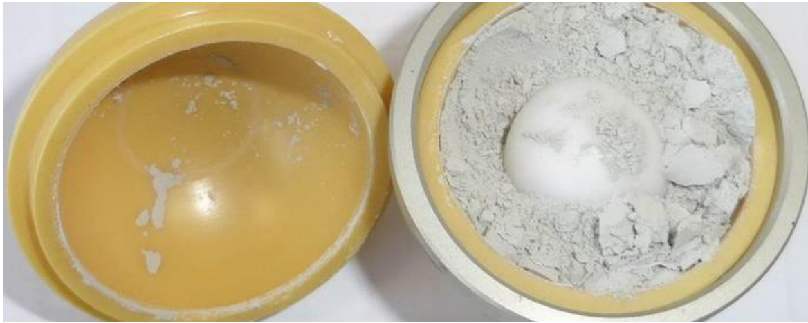
Sample 2555 after a total of 3 minutes of grinding. As seen in the lid of the bowl, sample is not sticking that strongly.
