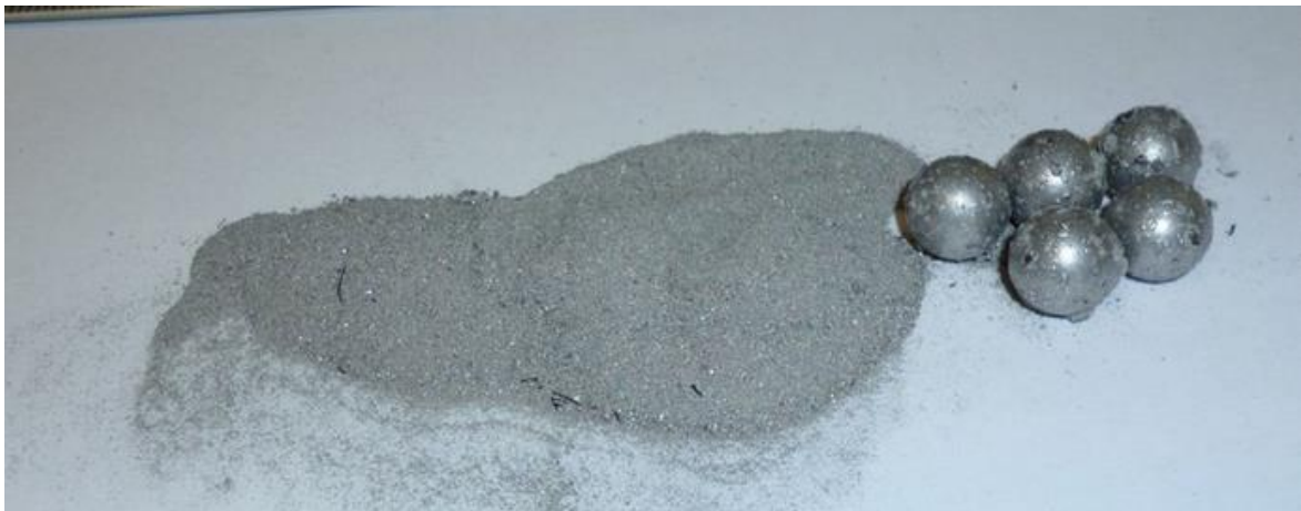
Emptied bowl after 5 minutes. The sample become ground, compressed sample is still sticking to the 10mm Ø zirconium oxide balls (formally white).
