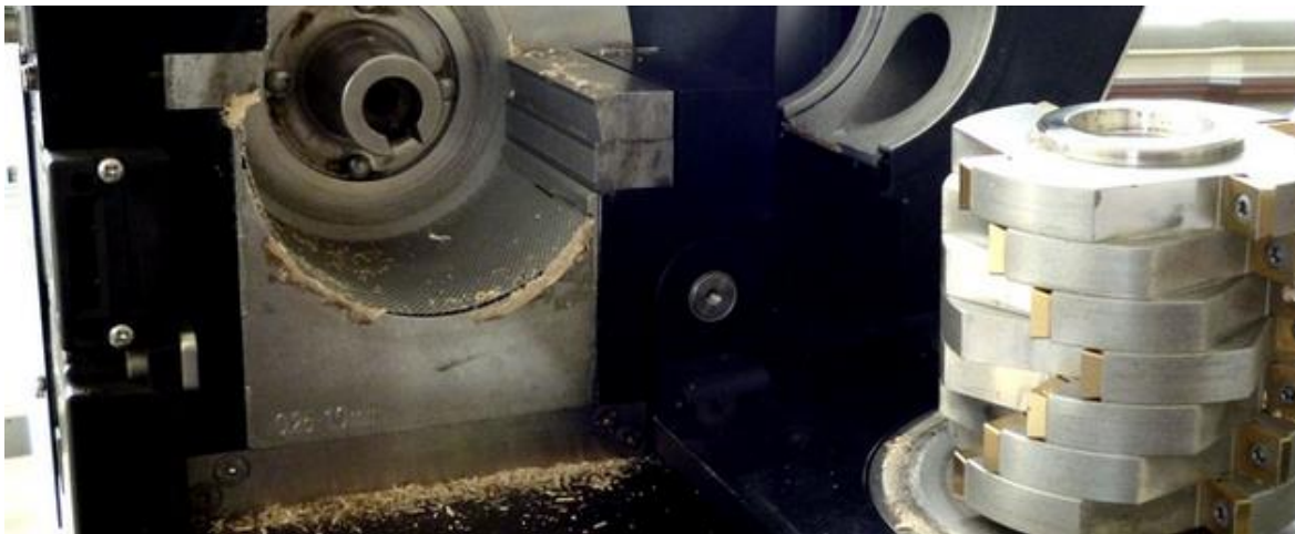
Grinding chamber after 2:45min. The very small amount of residue can be removed easily with a vacuum cleaner and a soft brush.
