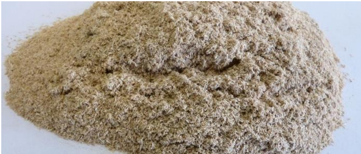
Sample after grinding with 0,5mm sieve cassette. Pieces up to 3-4mm length can be found afterwards.
